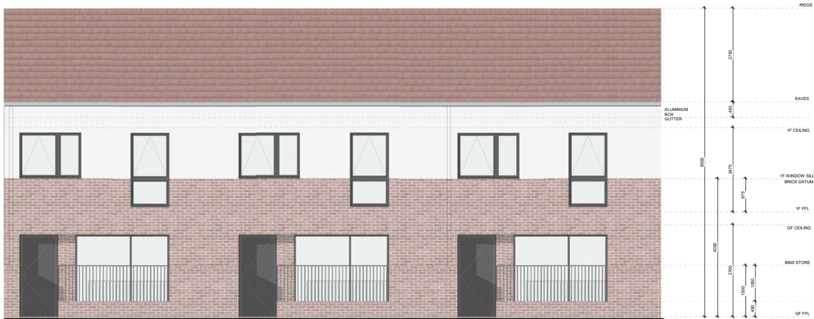
HOUSE H1 TERRACE - MATERIALITY - FRONT ELEVATION 1 : 50
