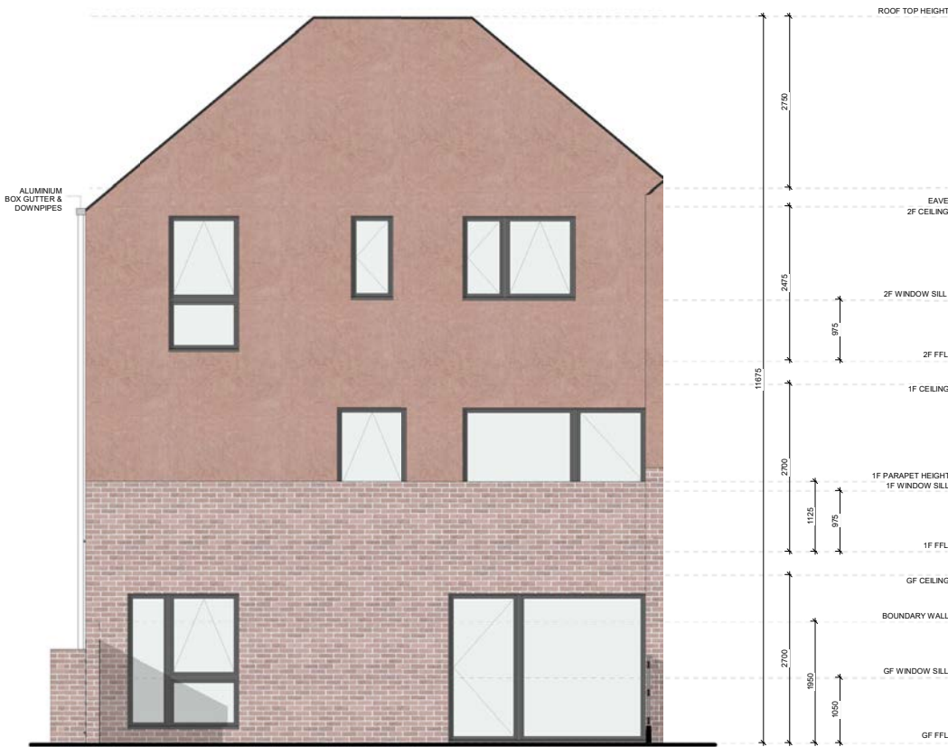
DUPLEX D1 - MATERIALITY - REAR ELEVATION 1:50
